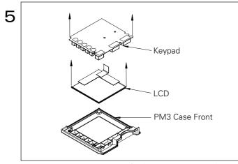
Remove rubber keypad and LCD from the PM3 case front.
