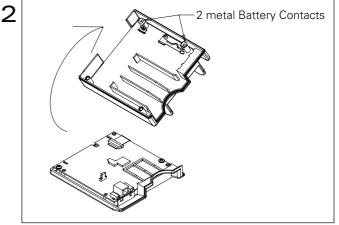
Remove case back. Note the position of the two metal battery contacts.
