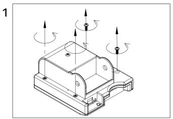
Unplug all wires and remove the PM3 from the indoor rower. Loosen the four PM3 case screws. Do not remove the two left screws
