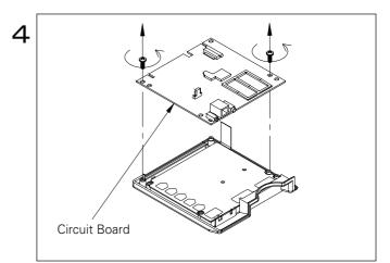
Remove the two Phillips head circuit board screws and remove the circuit board.
