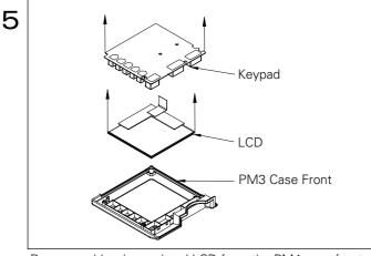
Remove rubber keypad and LCD from the PM4 case front.
