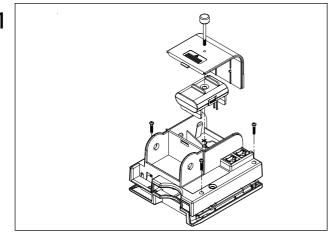
Unplug all wires and remove the PM4 from the indoor rower. Remove the battery door fastener and remove the battery pack (shown) or D cell batteries. Remove the four PM4 case screws.
