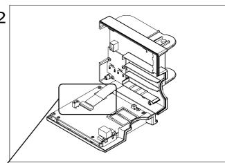
Carefully separate the case back from the case front, noting the position of the metal battery contacts.
