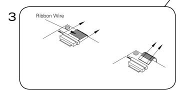
Detach the two flex cables from their sockets on the circuit board:
